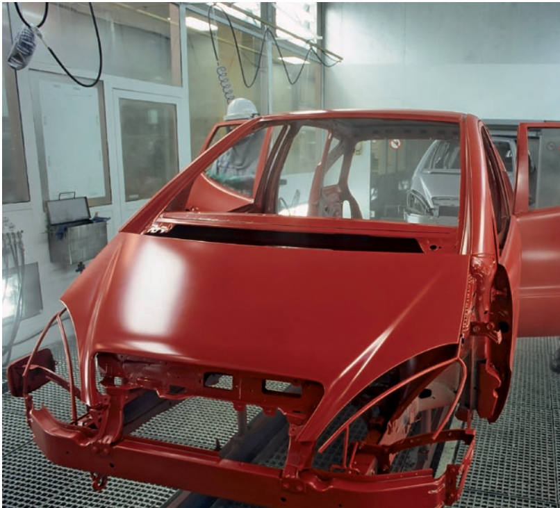
Car body after the painting process
