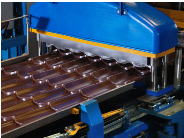
Figure 3: Cold forming of roof coverings
