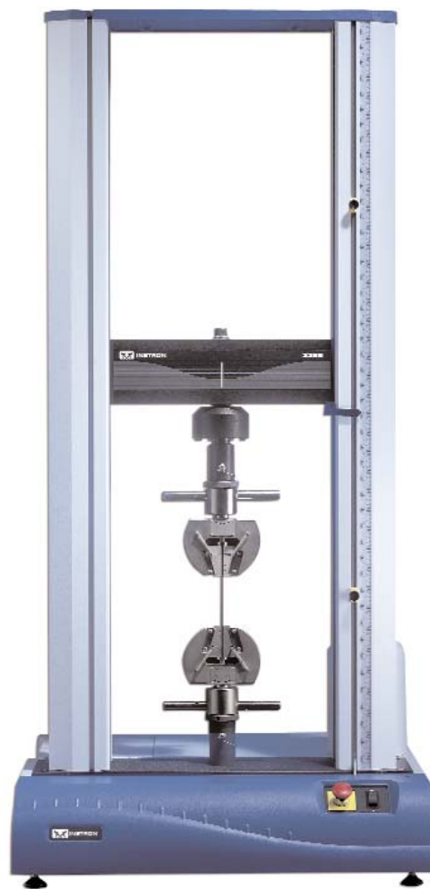
▲ Instron model 3369, in cobalt blue, configured for ASTM D 638, performing a plastic tensile test
