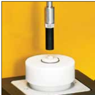
TA-DSJ F Dough Stickiness Fixture is standard test for measuring dough stickiness; important for processing raw dough. Fixture Base Table required.
